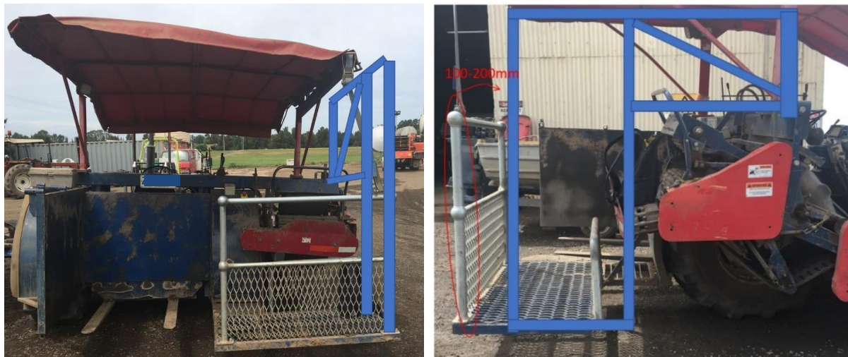
Figure 14 Example Rigid Platform Structure
