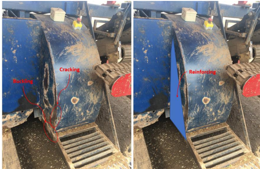
Figure 15 Cracking and reinforcing of rear wheel guard
