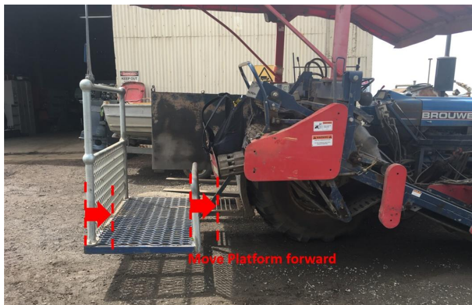
Figure 11 Reducing the Length of the Stacking Platform
